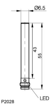
Inductive Sensors BES 516-371-S49-C D6.5 x 55 normally-open Sn=1,5mm shielded
